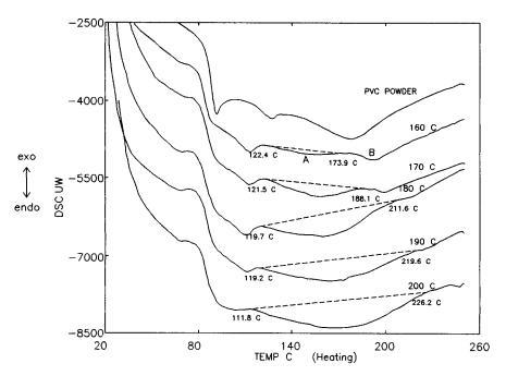
Figure 2 DSC thermal analysis curves of PVC compounds processed in a Haake Torque Rheometer at rotor speed = 60 rpm, TTQ = 10 kg-m-min, and various temperatures.<sup>4</sup>
