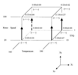
**Figure 5** Determination of the main effect of rotor speed  $(X_2)$  of PVC/5phr CPE/0.3phr OPE blend.
