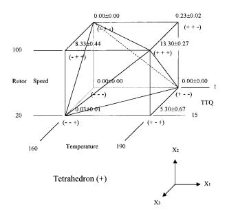
**Figure 8** Determination of the temperature vs TTQ interaction effect  $(X_1 \text{ vs } X_3)$  of PVC/5phr CPE/0.3phr OPE blend.
