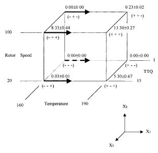
**Figure 4** Determination of the main effect of temperature  $(X_1)$  of PVC/5phr CPE/0.3phr OPE blend.
