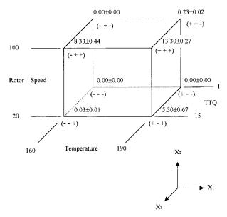
**Figure 3** Diagrammatic representation of the observed yields (heat of fusion: mJ/mg) and the standard ordering of experiments of PVC/5phr CPE/ 0.3phr OPE blend.
