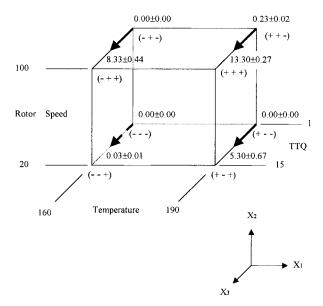
**Figure 6** Determination of the main effect of TTQ  $(X_3)$  of PVC/5phr CPE/0.3phr OPE blend.
