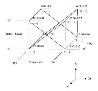
**Figure 7** Determination of the temperature vs. rotor speed interaction effect  $(X_1 \text{ vs } X2)$  of PVC/5phr CPE/ 0.3phr OPE blend.
